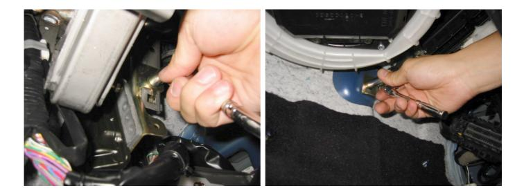
The ECU should come down easily with the bracket. Remove the bracket from the ECU and put all the nuts back onto the bracket. The ECU is now ready to be sent in for Flash Programming. These are all the parts you should have left over for the removal of the ECU.
