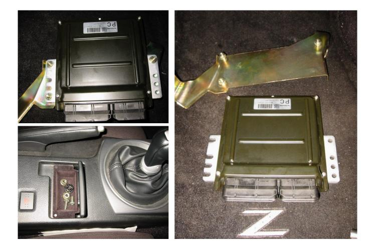
Installation is in the reverse order. After the ECU is re-installed there is no need to reset the ECU.
