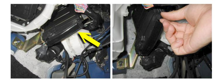
There are 2 nuts remaining until the ECU comes out. Look up towards the ECU and you will see a 10mm nut and another one towards the firewall. Remove them and put the nuts in the tray behind the shifter. (Pictures below)
