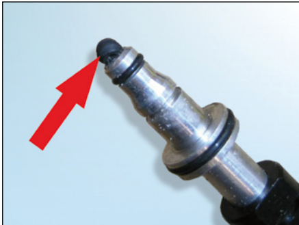
Image 4: If the old seal is not removed, it can get pressed into the CSC and block the tube.
